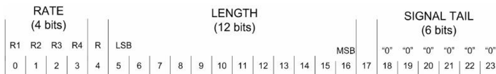
Fig. 2.2: ERP-OFDM PDU header for 802.11a.
