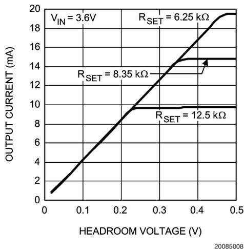
**FIGURE 4.  $I_{LED}$  vs  $V_{HR}$
