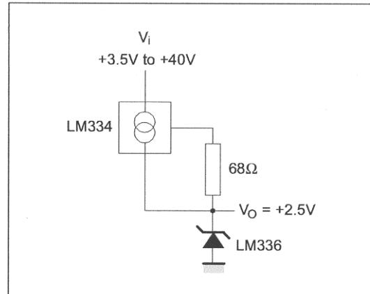
**Figure 5 :** Precision Power Regulator with Low Temperature Coefficient
