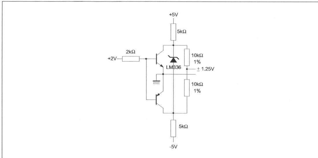
**Figure 9 : 5V Buffered Reference**
