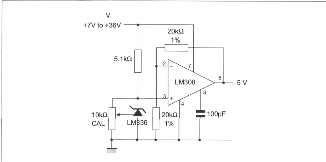
**Figure 10 : Low Noise Buffered Reference**
